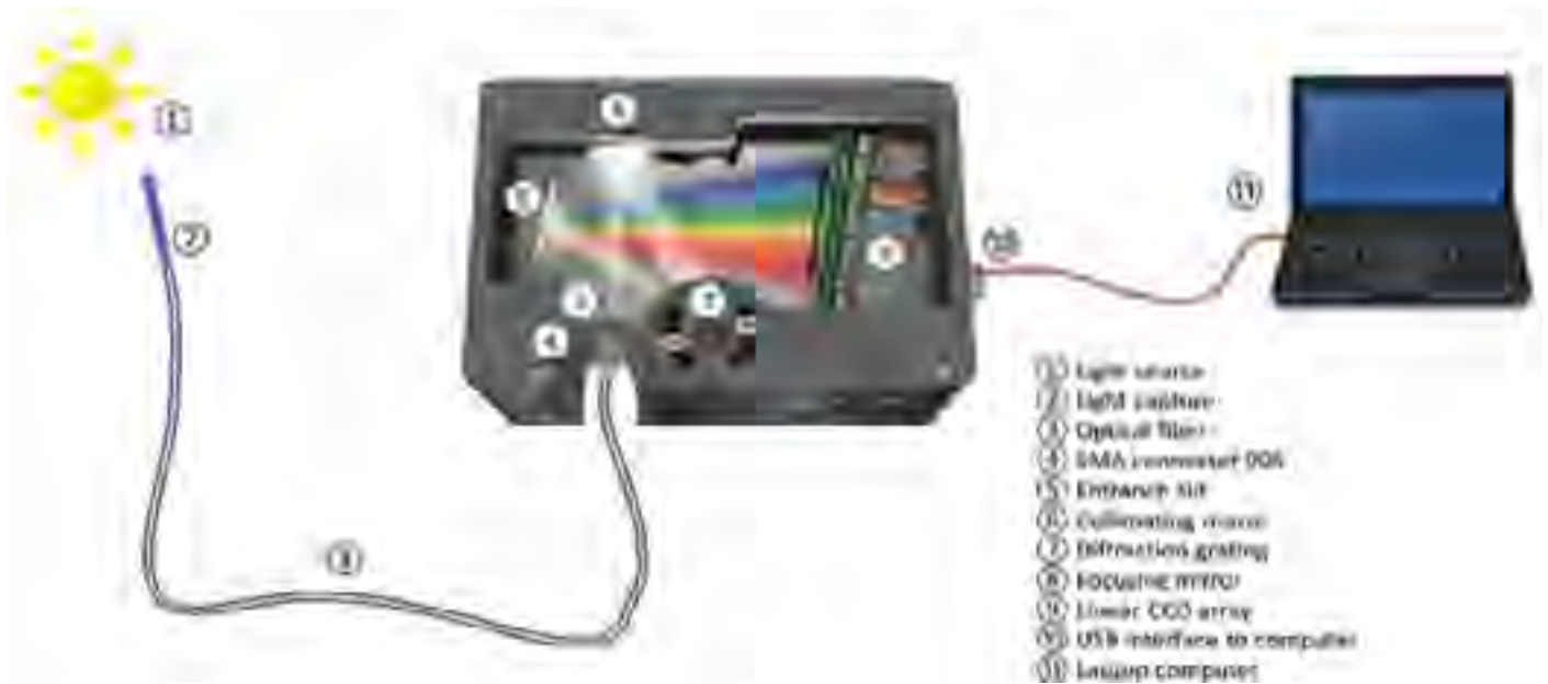
Figure 3. Operating diagram of an optical spectrometer such as the one used in this study [41].
