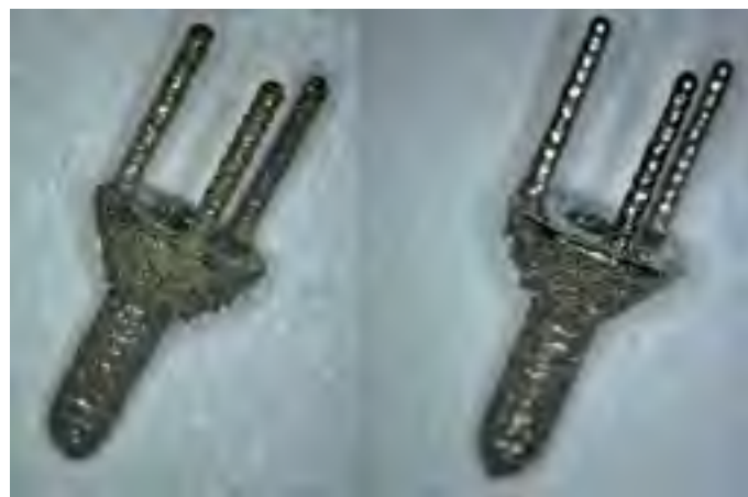
Figure 3. Figures 3A (left) is the implant abutment before DET and 3B (right) is the abutment after DET. Maximum width of abutment is 4.5mm
