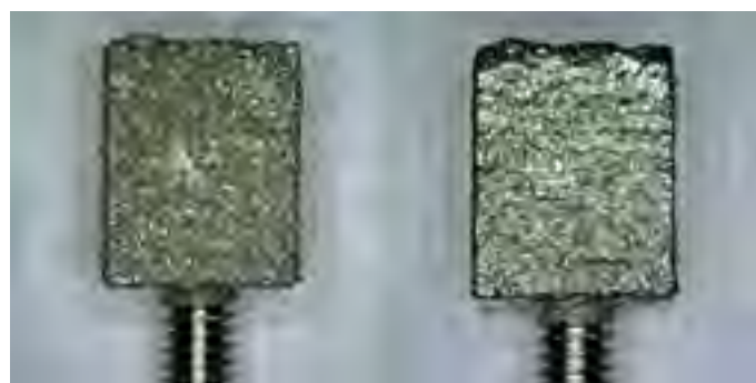
Figure 2. Figures 2A (left) is the implant abutment component before DET and 2B (right) is the component after DET. Width of component is 4.5mm.
