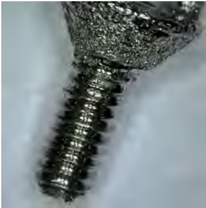
Figure 5. Abutment threads. Width of shaft is 2.1 mm.
