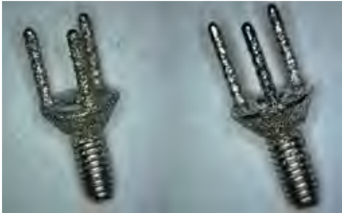
Figure 4. Figures 4A (left) is the finalized implant abutment before DET and 4B (right) is the abutment after DET. Maximum width of abutment is 4.5mm.
