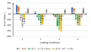
Figure 3. Error indices I for 34Cr4 steel alloy
