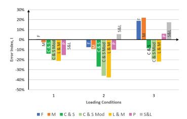
Figure 2. Error indices I for 42CrMo4 steel alloy
