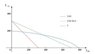
**Figure 1.** Variation of the fatigue resistance limit in pure torsion,  $t_{-1}$ , with the mean shear stress  $\tau_m$ .
