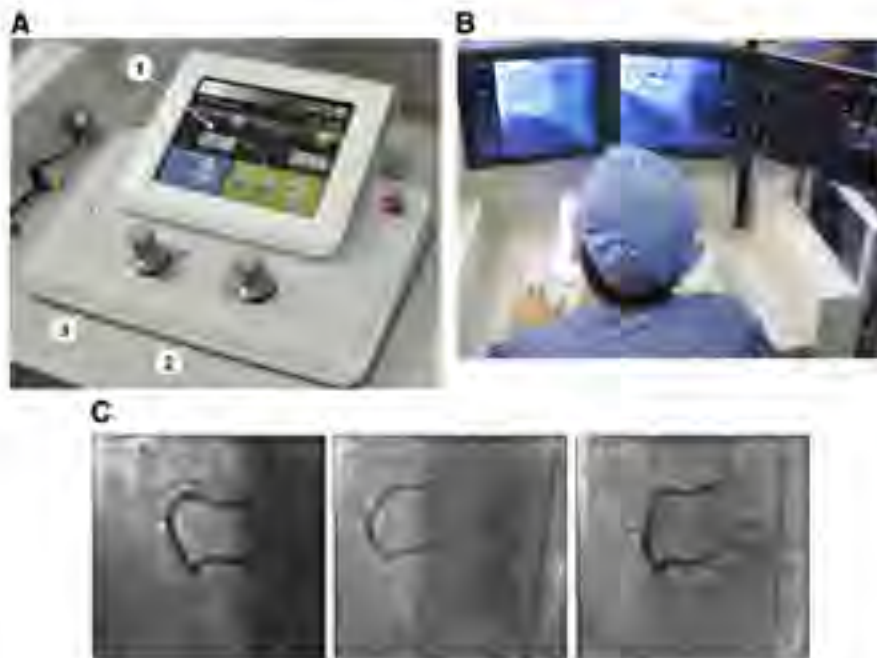
Figure 2. CorPath 200 System Console (A) Representative picture of the control console: 1—touch screen controls; 2—guidewire joystick; and 3—balloon/stent catheter joystick. (B) The operator seated at the interventional cockpit with control console for manipulating percutaneous transluminal coronary angioplasty devices and the angiography and hemodynamic signs monitors positioned at his eye level. (C) A guidewire and then a 2.5- 9-mm balloon were advanced through a proximal posterior descending artery lesion with the robotic angioplasty arm to perform pre-dilation. A 2.5- 16-mm stent was delivered to the target lesion with the robotic system and deployed in a standard fashion.
