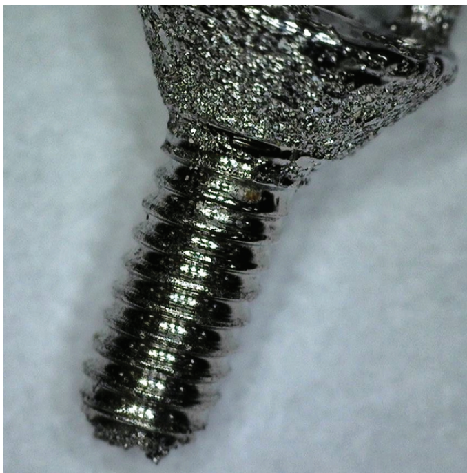
Figure 5. Abutment threads. Width of shaft is 2.1 mm.
